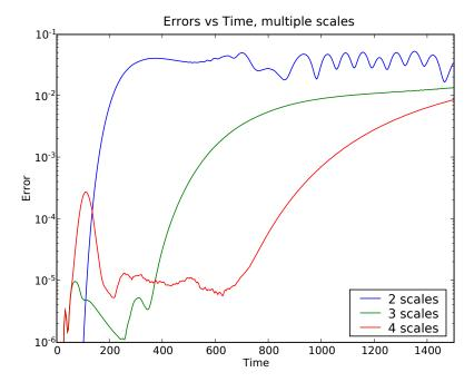
Figure 6: A graph of error (relative error, measured in  $L^2$ ) vs time for a test involving a long range potential. As predicted in section 4.1, the time that the simulation remains accurate increases with the number of scales.
